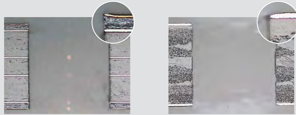
Cross sectional view through a printed circuit board, with unbrushed bore hole
