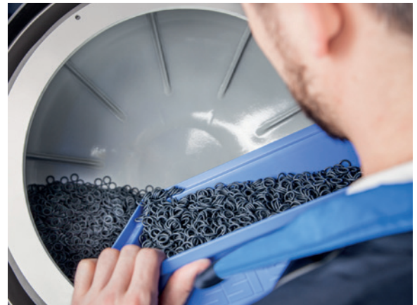
Loading of the drum with O-rings
