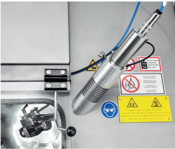
IR sensor for measuring the work piece temperature
